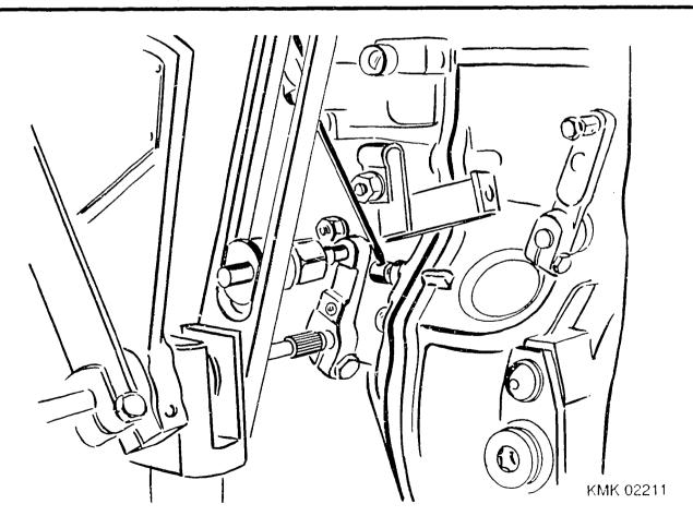
ADJUSTING IDLE AND SHUTOFF STOP
